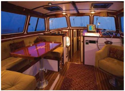
We took advantage of the lull in wind speed to do some full-throttle, full-lock turns. The aft steering station is a manual Whitlock unit, five turns from lock to lock. The inside steering station is hydraulic. With the hydraulic autopilot operating independently, there are three separate and redundant steering systems, with a manual tiller backup just in case you are having a really bad day on the water.
